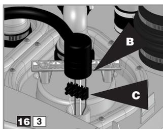
Unscrew the collar **B**. Remove the motor power wires **C** from the screw connector.
