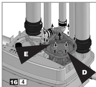
Remove the screws **D** from the inspection cover. Use the handle **E** to lift the motor carefully.
