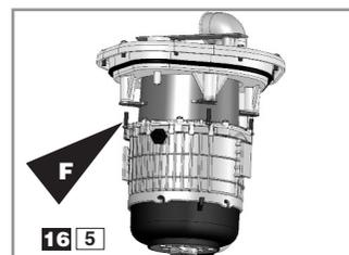
Please contact the service engineer. You can operate the lifting station in minimum configuration with just one motor. Remove the screws **F** of the faulty motor from the inspection cover.
