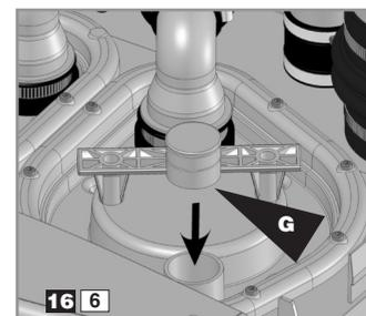
Put the inspection cover back in place. Reconnect the discharge pipe. Use the plug **G** to close off the motor cable outlet in the inspection cover. Fix using the hose clip **B**.
